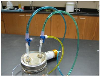
3. When the lines are free of  $CO_2$ , switch the valves to circulate air between the jar and the Licor.
