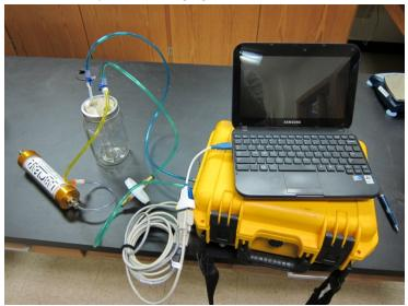
2. Set up the tubing as shown below. This will draw air from the soda lime canister and flush the lines of any CO<sub>2</sub>
