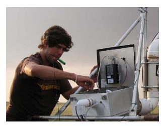
Fig. 3. Photograph of a graduate student working on a mobile mesonet rack. Mobile mesonet probes were used to acquire near-surface kinematic and thermodynamic characteristics of rear-flank downdrafts.
