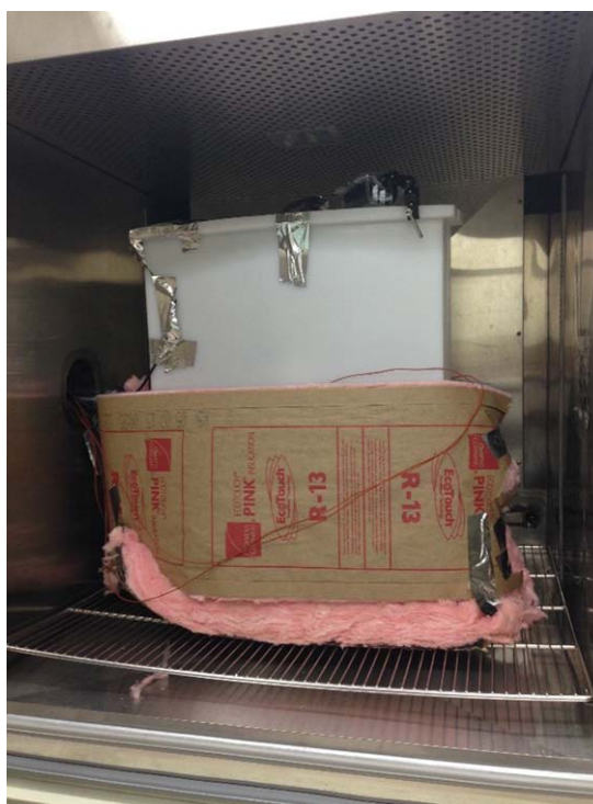
Fig. 2. Photo of the inside of the Tenney environmental chamber in between experimental runs showing the insulated polyethylene tank.
