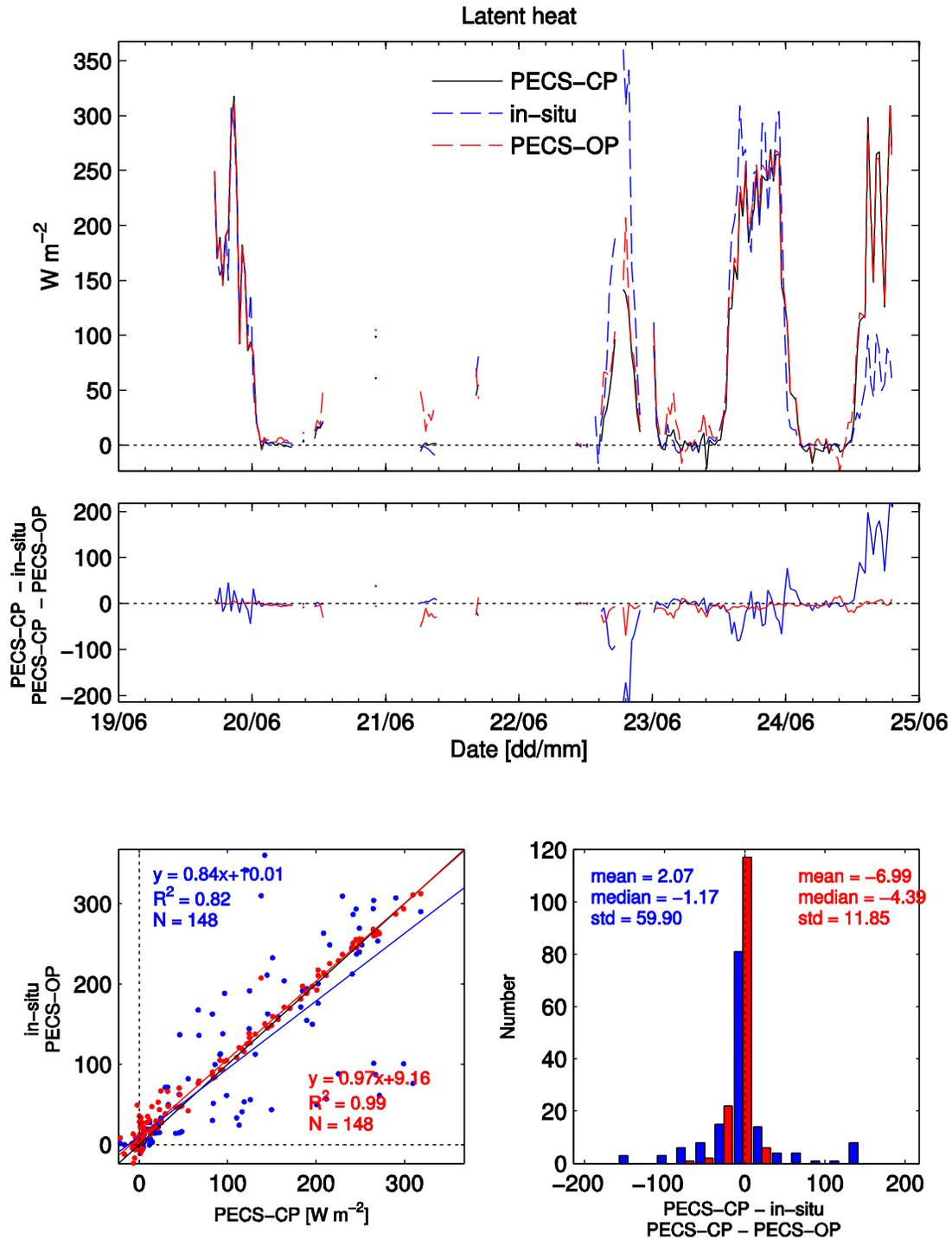
Figure - PECS open-path, closed-path and *in situ* latent heat fluxes.
