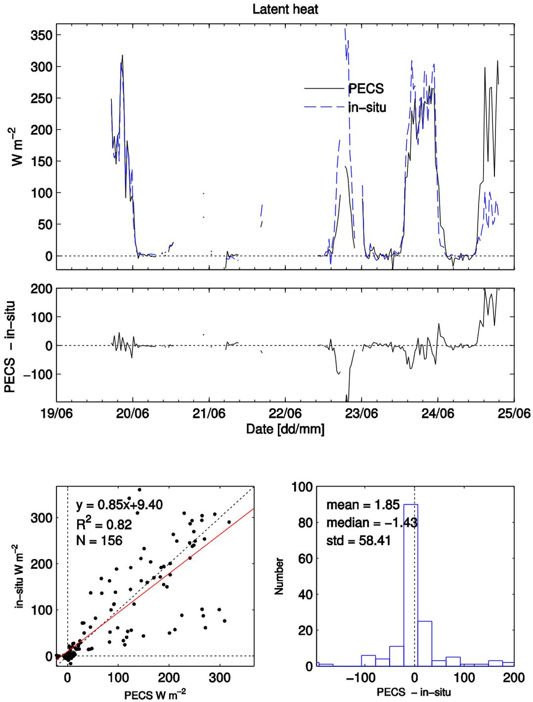
Figure - Closed path latent heat fluxes.
