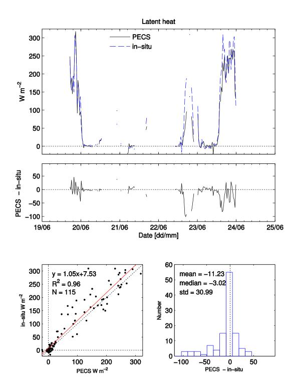
Figure – Closed path latent heat fluxes with points after 24 June removed.
